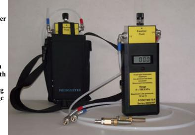
Suitable for Differential Pressure measurement across balancing valves, orifice plates, chiller etc. in waterflow systems.
